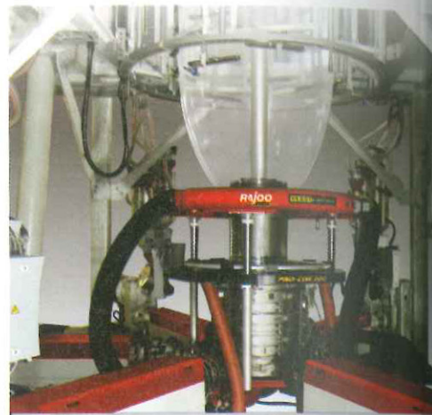
The PENTAFOIL all-PE 5-layer co-extruded blown film line from Rajoo
